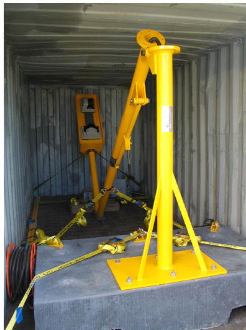
Fold-down block-mounted LVS ready for shipping in 20-foot container
